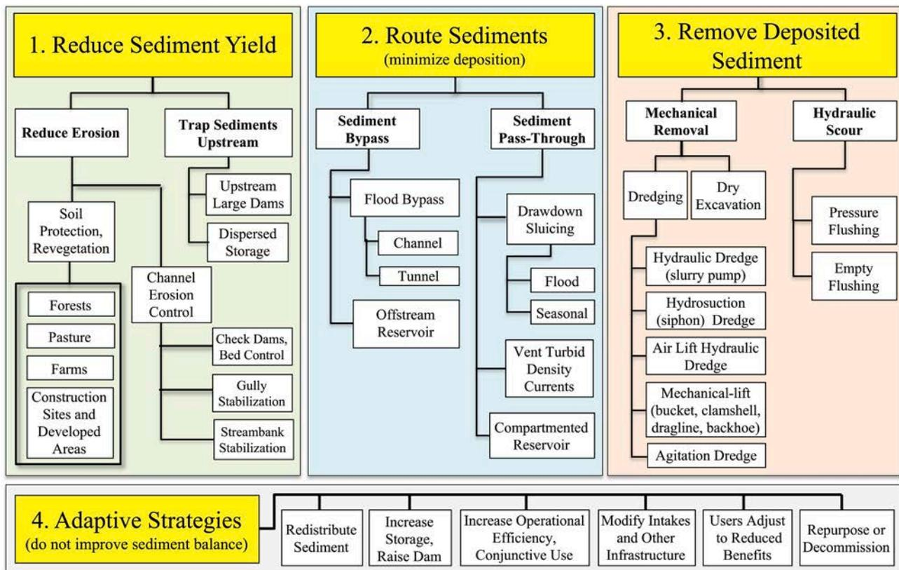
Fig. 7. Classification of methods to manage reservoir sedimentation (Morris, 2020).
