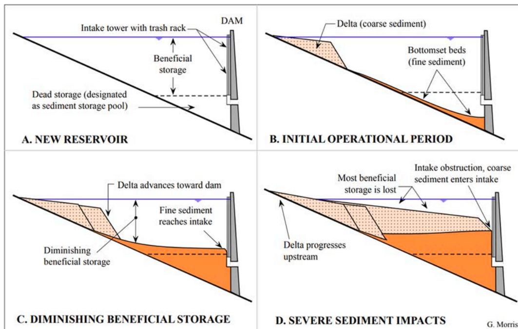
Fig. 4. Process of reservoir sedimentation. A) new reservoir showing zone of beneficial storage and the designated sediment storage pool; B) initial operational period with minimal sediment impacts, showing the deposition pattern for both coarse and fine sediments; C) significant sediment encroachment into the beneficial pool with substantial growth of the delta; and D) severe sediment impacts including loss of beneficial storage, intake obstruction and upstream progression of the delta.
