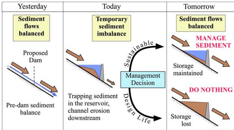
Fig. 1. Trapping sediment in a reservoir and releasing clear water downstream is neither a natural nor a sustainable option over the long term. Preservation of long-term reservoir storage capacity is a management decision and requires the downstream release of sediment to match natural inflows (Morris, 2020).
